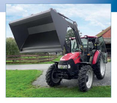
A hardened cutting edge (500 HB) protects against unnecessarily high wear. The design of the bucket results in a favourable centre of gravity close to the tractor or loader.
