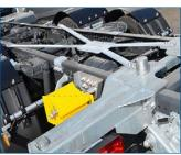
> on request, you can obtain our proven multi support beams for mounting e.g. hand-held extinguishers and tool boxes.
