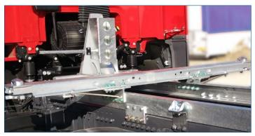
Like all other assemblies, the **middle support** consisting of two spacers is available to suit the respective system height. You will receive adapted components or additional height adapters. For height adjustments there is a additional hinged middle support.
